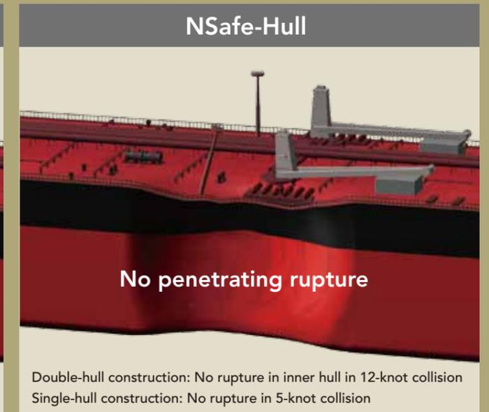
Double-hull construction: No rupture in inner hull in 12-knot collision
