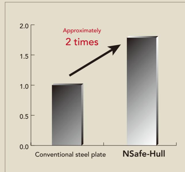
Critical striking ship speed for penetration, normalised by value of case with conventional steel.
