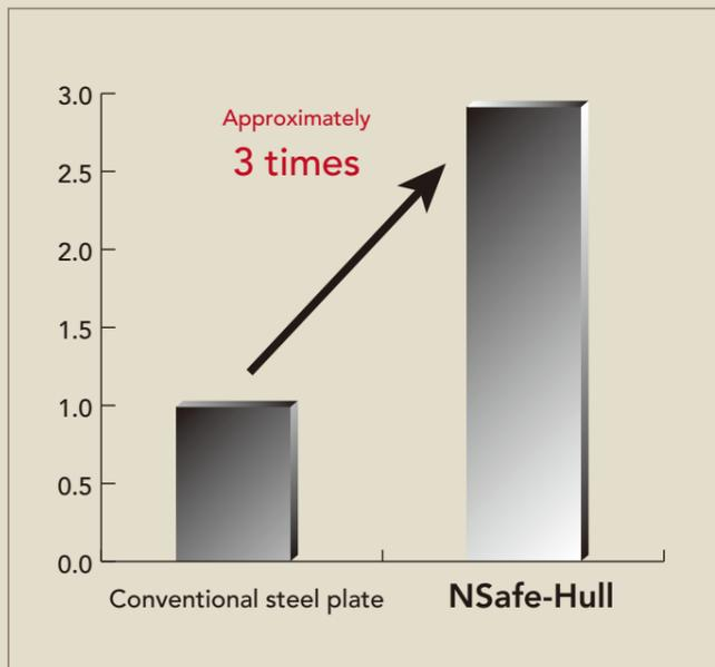
Absorbed energy by struck ship, normalised by value of case with conventional steel.
