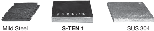
Photo 3.1 10.5% Hydrochloric Acid, 60°C, 72 Hrs
